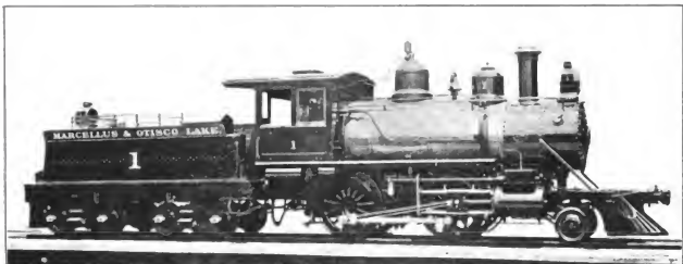
Fig. 23. Four-Coupled (2-4-0) Locomotive. Built by the Baldwin Locomotive Works for the Marcellus & Otisco Lake. Cylinders 17 in. x 24 in., Working Steam Pressure 160 lbs. per sq. in., Total Heating Surface 1,012.4 sq. ft., Diameter of Drivers 56 in., Weight on Drivers 71,160 lbs., Total Weight 84,460 lbs.
